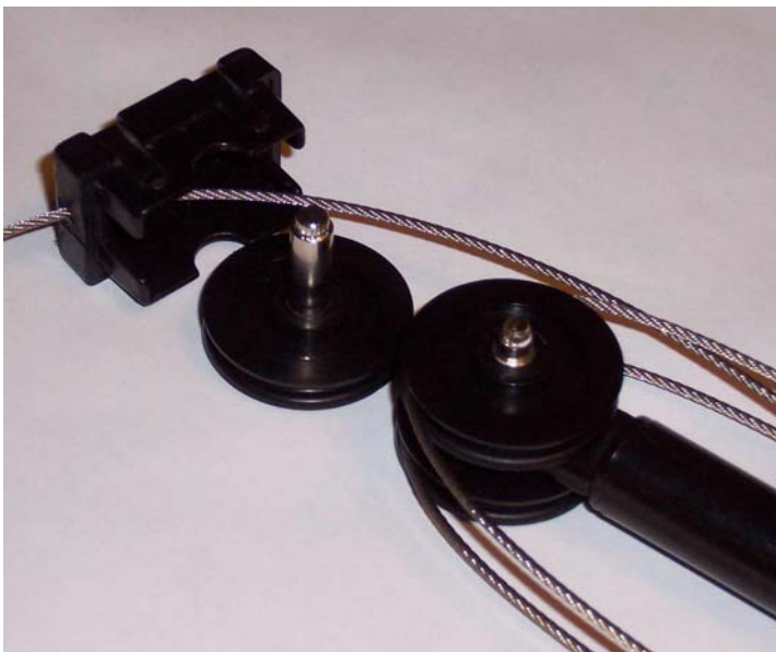
Pulley system at top of cable closer
