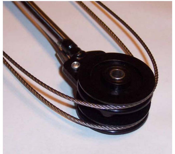
Pulley system at bottom of cable closer
