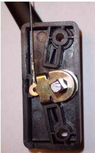
**Exterior handle with cable correctly positioned and cable attached (Step 6)**
